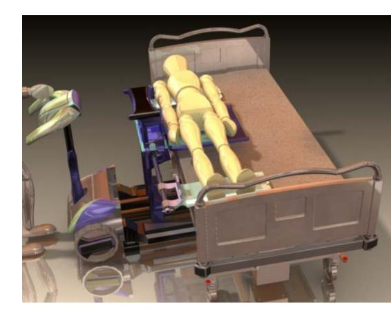
The hospital staff could use the device for lifting of patient in order to make necessary hygienic procedures or for transportation of the patient from the hospital transport bed to the hospital or operation bed and vice versa.
