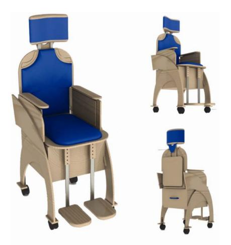
The result was a chair with wheels for use only at home, with many adjustable parts for following the changes in body dimensions: footrests, armrests, backrest, headrest etc. The ranges of adjustability were determined with an analysis of anthropometric measurements for children of different ages.
