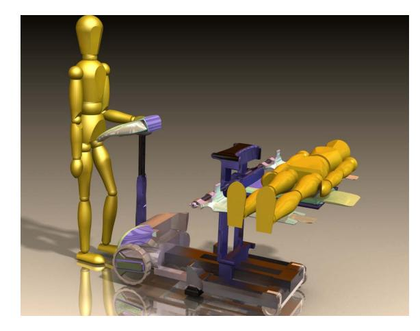
The student lgor Ivanovski made an innovative design of a device that could be used for lifting of patient in horizontal position and for his transportation in horizontal or seating position.
