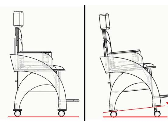
The seat is designed with possibility to change the angle of the backrest in order to obtain relaxed position. The child could be positioned on the seat with extra equipment as a medical treatment for the posture.
