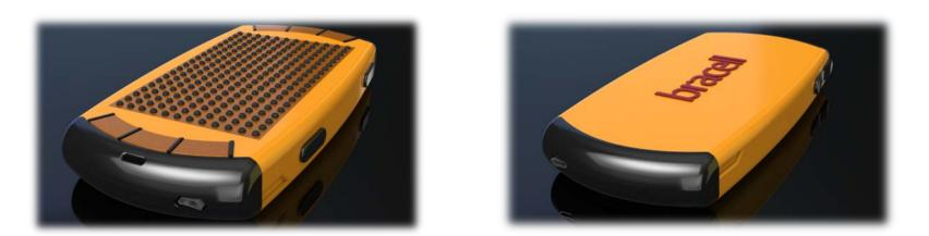
The screen for reading of messages is a matrix of mechanical dots that could move up and down across the flat surface of the front side of the phone in order to present different Braille sign. The signs could be recognized by the user when he moves his fingers across the screen. Each sign is consisted of 2 columns with 3 dots. The screen is designed for presentation of text in 4 rows with 10 signs per row.
